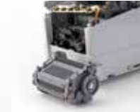
Remove Roller Unit without using any tools.
