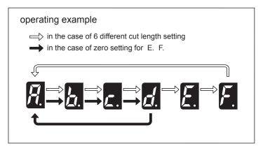
Please take the following procedure when using P MODE or L MODE. After setting Programing Function, press SELECT BUTTON and P will be displayed.
